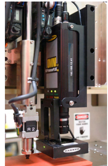
Camera mounted on pickup assembly
