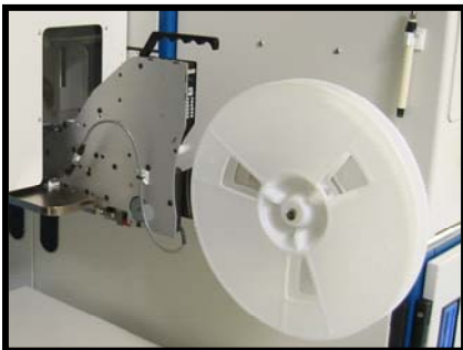
Tape & Reel Input Hover-Davis mechanisms
