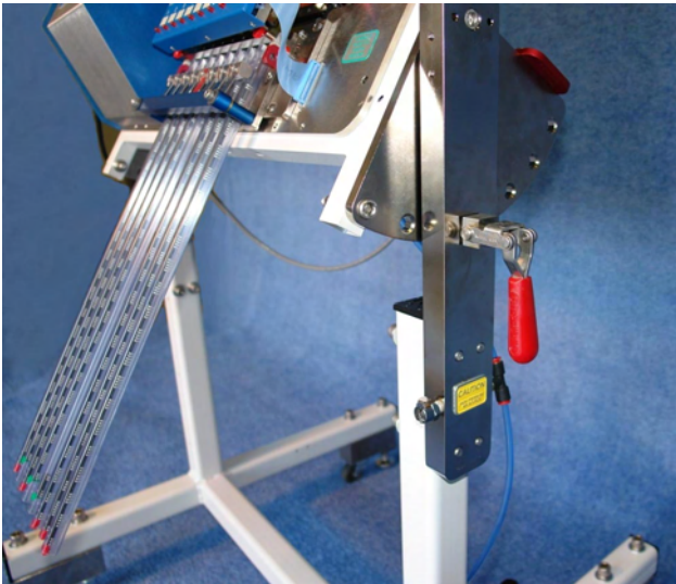
Stand with frame tilt angle adjuster
