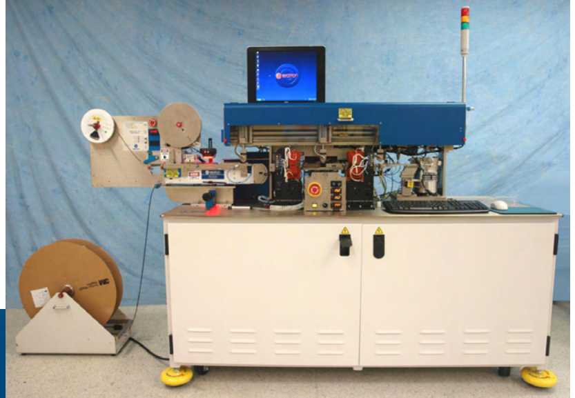
Bowl feeder on Model 900 with MEMS magnetic & thermal testing
