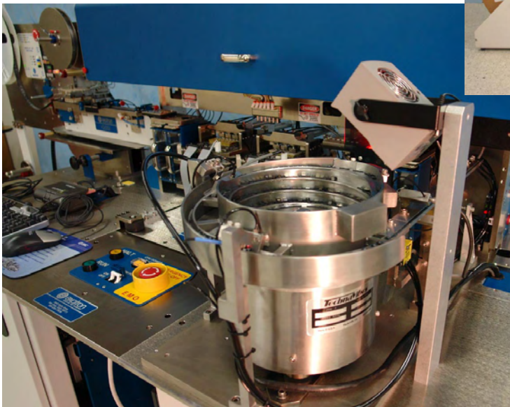
Bowl feeder on Model 900 with MEMS vibration testing
