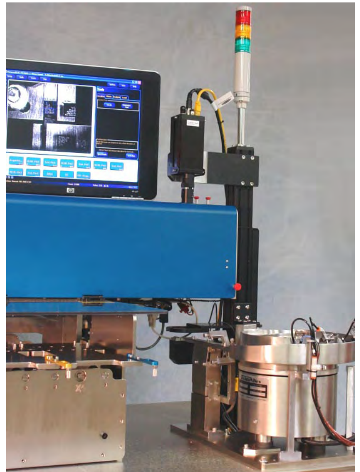
Bowl feeder with machine vision at dead nest pickup site
